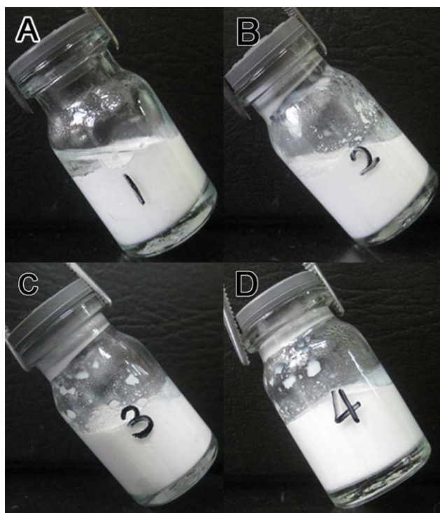
Figure 9. Photographs of the WBPU/PS emulsion at the polymerization time of (A) 1 h, (B) 2 h, (C) 3 h and (D) 4 h when the St/WBPU feed ratio was 10/1 (wt/wt) and St/DVB = 98/2 (wt/wt). The polymerization temperature was 70°C.
